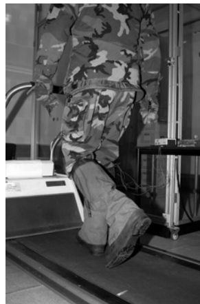
Figure 1: Test drill on a treadmill in a climatic chamber at -18°C.
